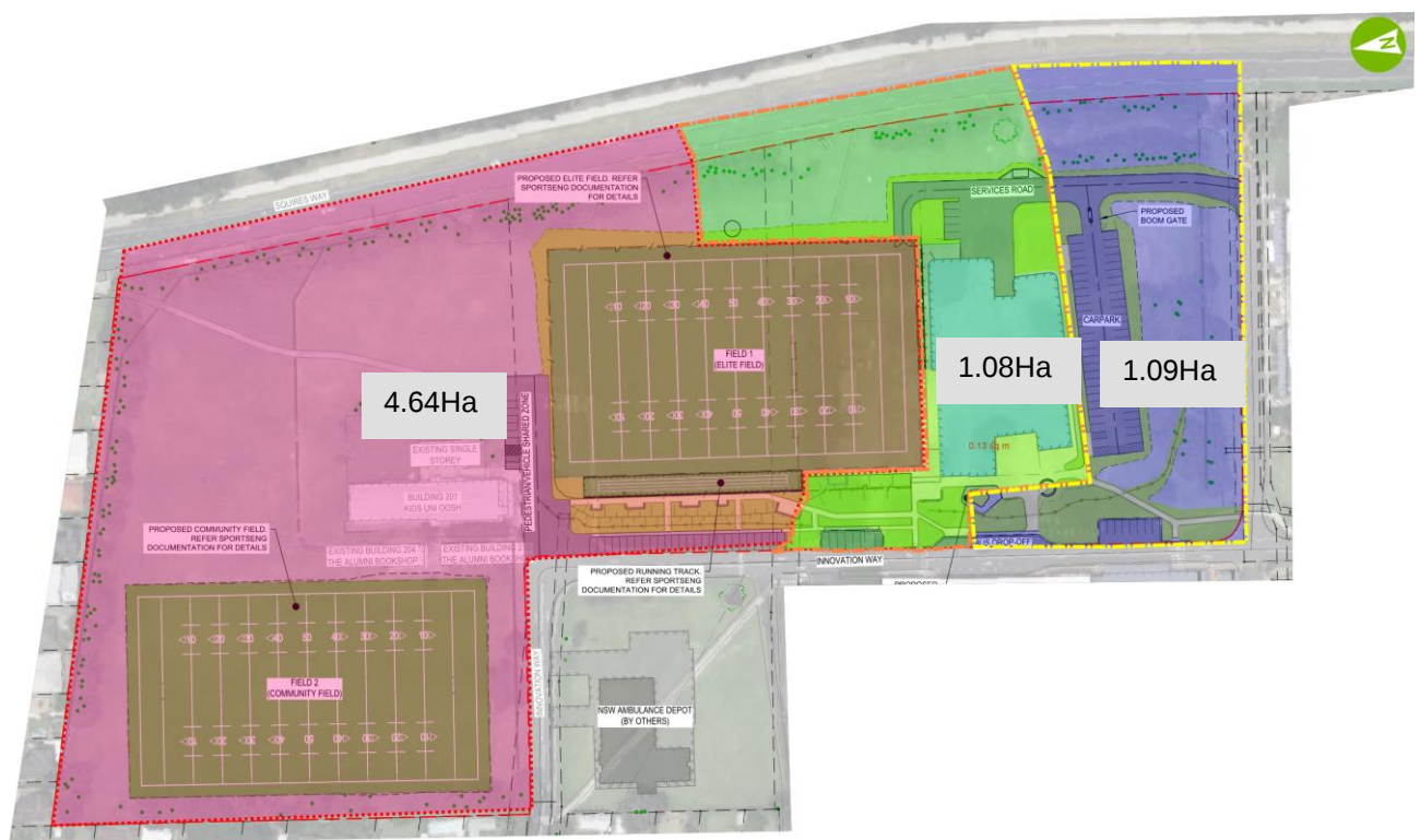
Figure 8-3 Site Only Post-Developed Catchments
